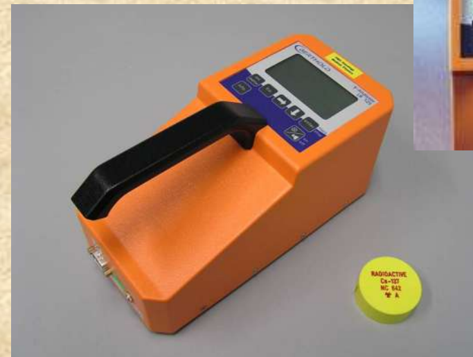
Portable MCA with detachable Cs-137 check source
