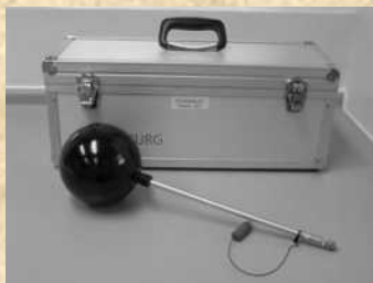
1-litre Ionization Chamber (reference)
