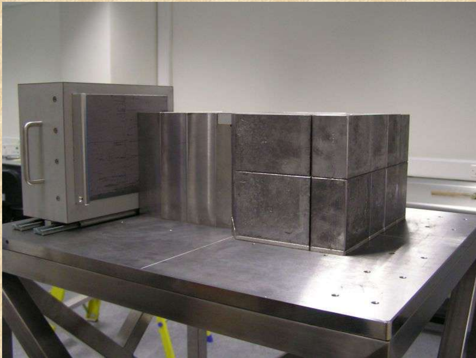
From left to right: 4-inch lead door, collimator and Cs-137 storage safe.
