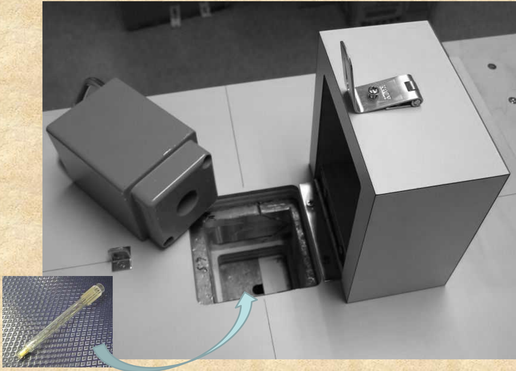
Top view of the irradiator. 2 tubes of Cs-137 each of activity 290MBq (2007) are inserted into the hole. On the top, it is encapsulated by a lead cap
