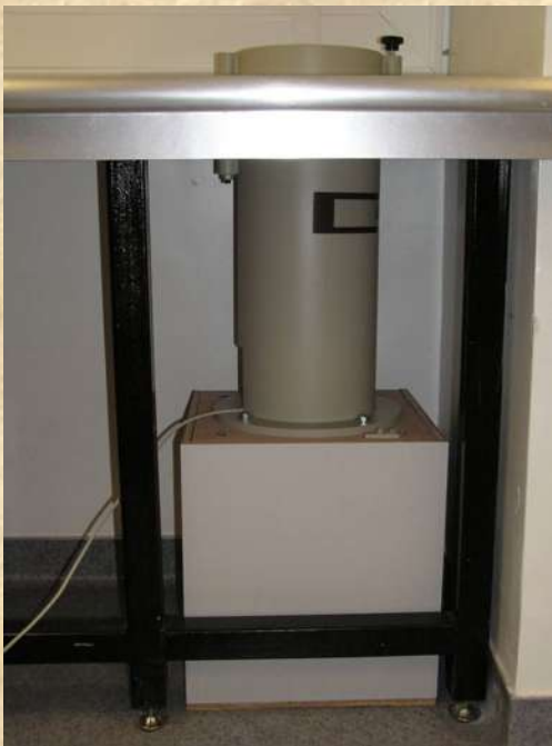
MCA (NaI) for wipe/contamination test
