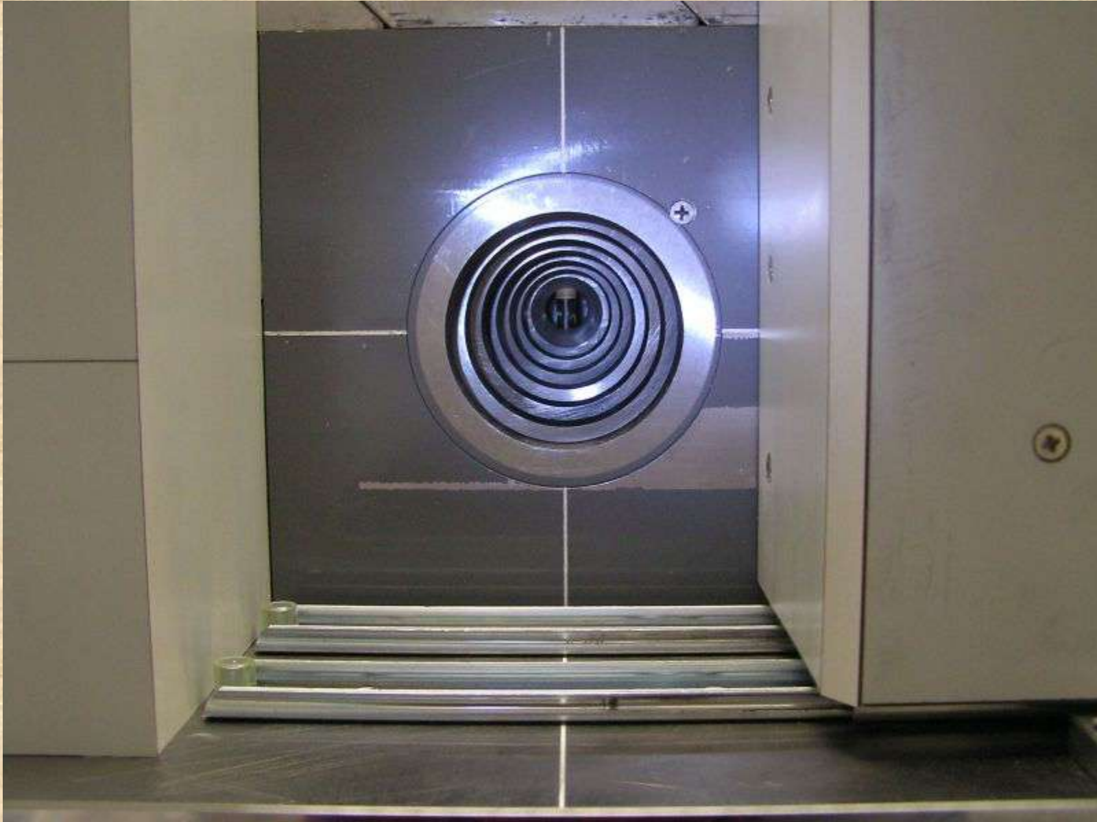
Front view of the irradiator with a dummy source.
