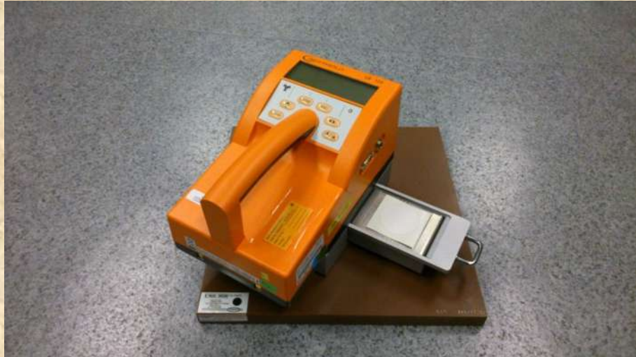
Contamination monitor with wipe sample Drawer (for alpha/Beta/Gamma measurement)
